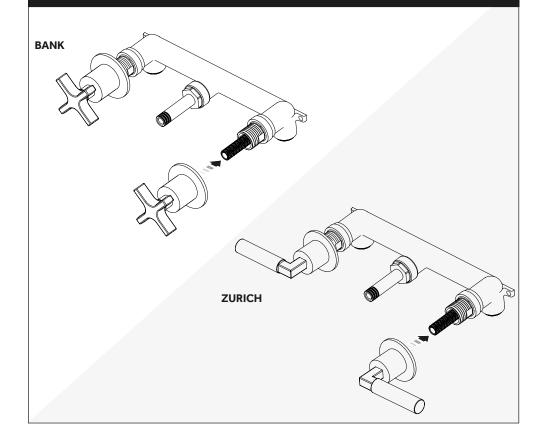
1. Installing the Bank and Zurich handles onto the wall mounted products is a simple operation. The handle assembly is screwed onto the exposed flow sleeve until the backplate sits against the wall.
